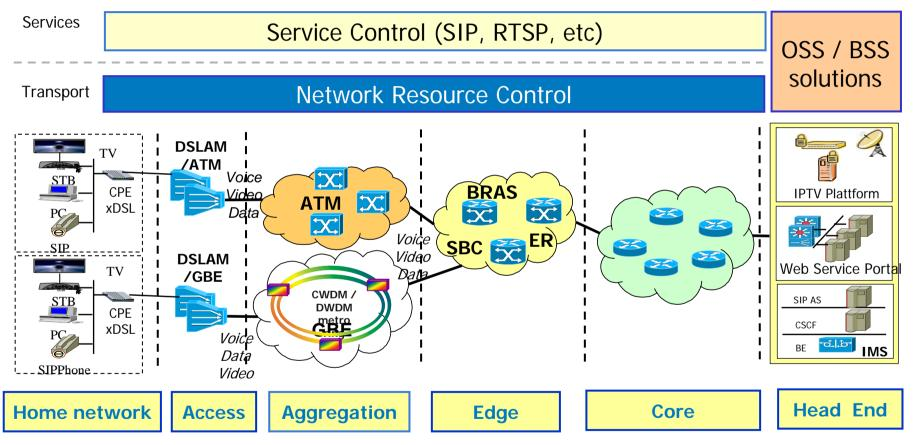
Multi-technology access: DSL, FTTP, CATV, UMTS, WLAN, WIMAX/WIBRO, PSTN Converging to IP Diffserv and MPLS in core (and aggregation)
